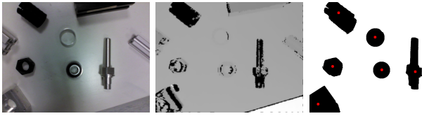
Fig. 8. Left: An example image from the dataset, displaying multiple RoboCup@Work objects. Center: The corresponding depth image. Right: Imperfect segmentation mask obtained by the current RoboCup@Work software. Manually labeled pickup positions marked in red.
