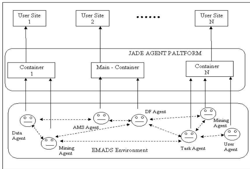
Fig. 2. EMADS Architecture as Implemented in Jade
