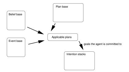
• A plan is selected, its goal is the current intention, and the plan is pushed onto the intention stack.
